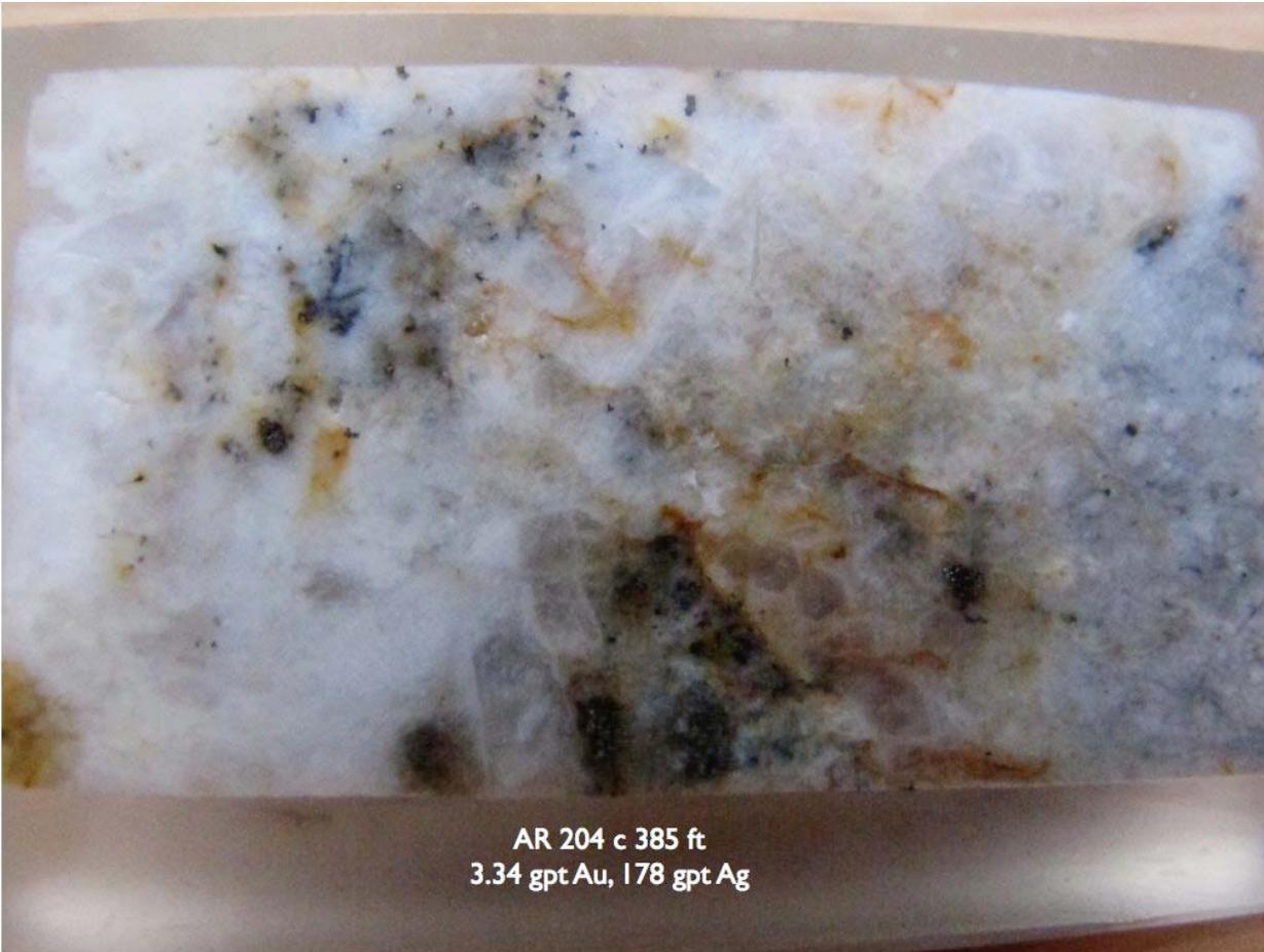
Figure 7-5: Cut core from hole AR 204c at 385 ft (272 ft vertical depth), showing partial oxidation (brown limonite) in the Moss vein
