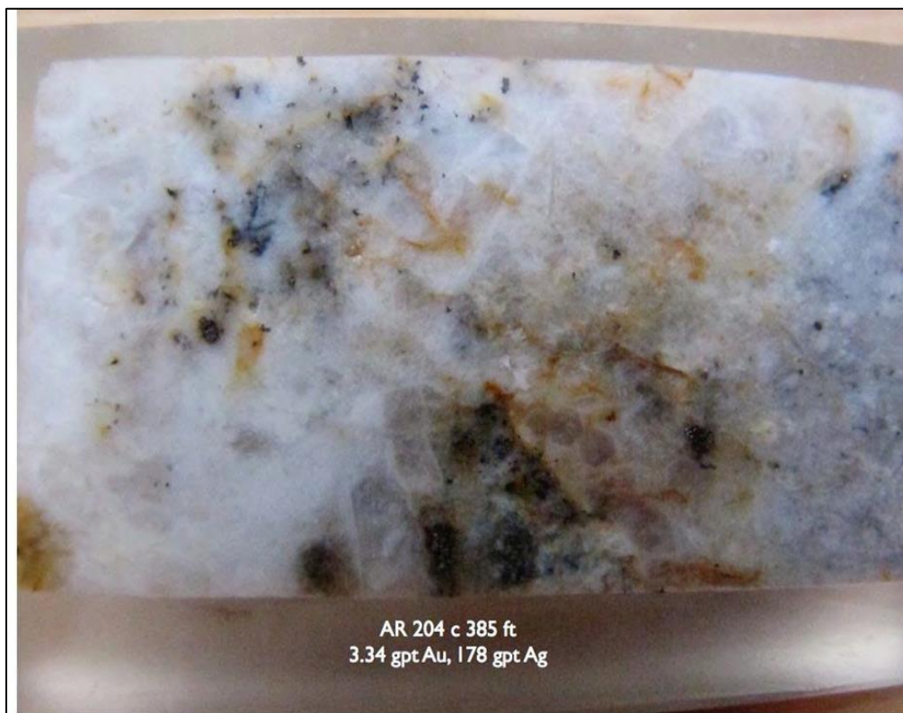
Figure 7.6 Cut Core from Drill Hole AR204C at 385 ft Downhole (272 ft vertical depth), Showing Partial Oxidation (brown limonite) in the Moss Vein
