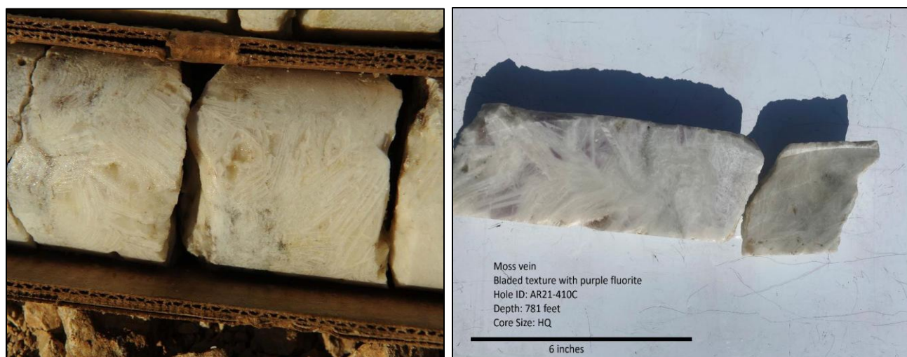
Figure 8.1 Examples of bladed calcite partially replacing quartz (evidence of boiling) in HQ- diameter (2.5”) diamond core drill holes: Right a) AR-165C at 213 ft; Left b) AR21-410C at 781 ft (with purple fluorite)
