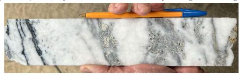
Figure 7-8 SVS Mineralization Overprinted on QS Vein, Mina Francisco, Drillhole LC22-549, Assayed 8.7 g Au/t and 49.2 g Ag/t
